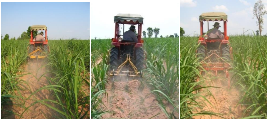
Figure 8: The comparative testing between second prototype, third prototype and local made spring tine
