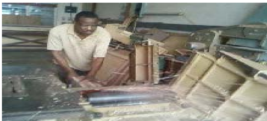
Fig 5; Planing beams after lamination
