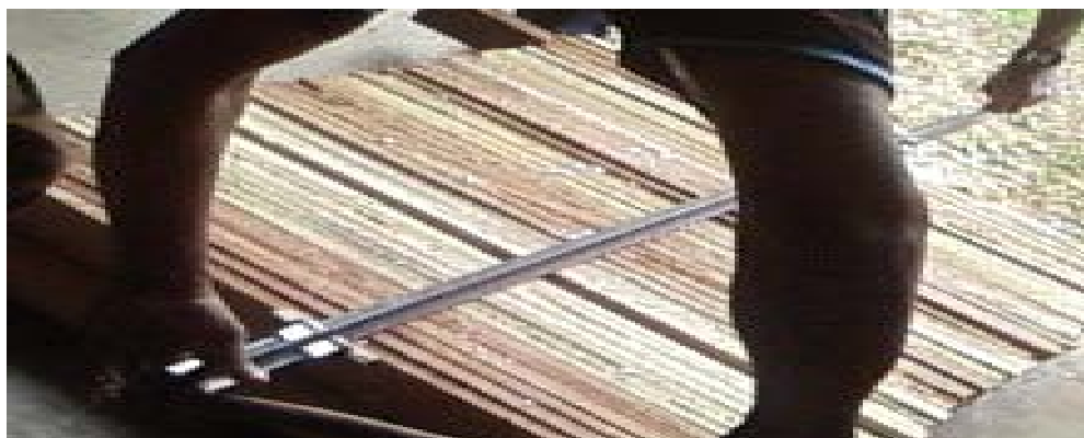
Fig 4; Clamping wood together after applying glue
